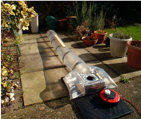
Photo 1. General view, fan unit at front, air outlet at far end, wooden load on top of tube.
